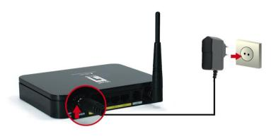
**4.** Press the Power ON switch on the rear of the router.
