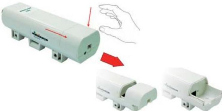
2. Plug Cat.5/5e/6 cable into the RJ-45 port.
