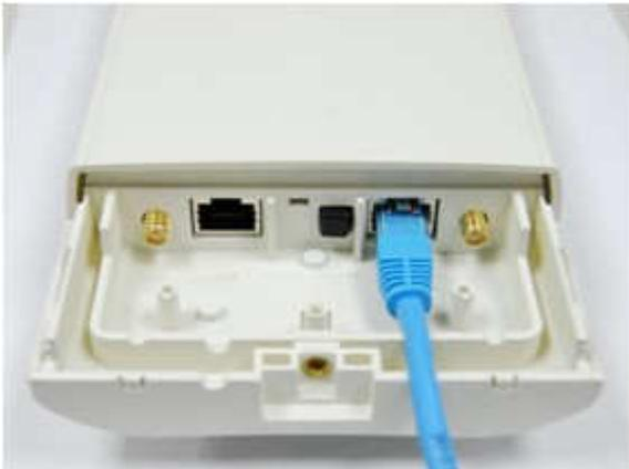
3. Power on the CPE by press the black PWR button beside the LAN 1 Ethernet port.
