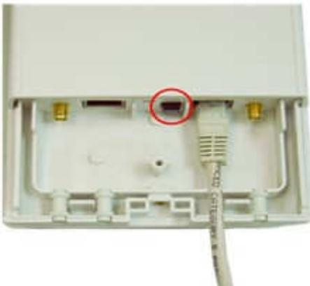
4. Attach and fasten the removable cover to the bottom of the unit with the screw
