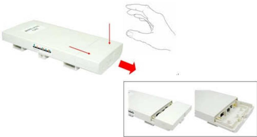
2. Plug Cat.5/5e/6 cable into the RJ-45 LAN1 port. Do not use the RJ45 LAN2 port.
