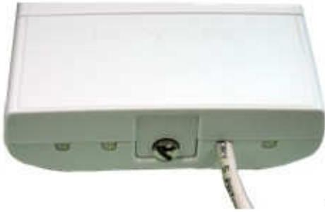
5. Plug the power cord into the DC port of the PoE injector
