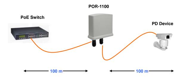
\*\* Note: If the Ethernet cable is not standard CAT5 cable, the POR-1100 may be working for shorter length than 100 meter.
