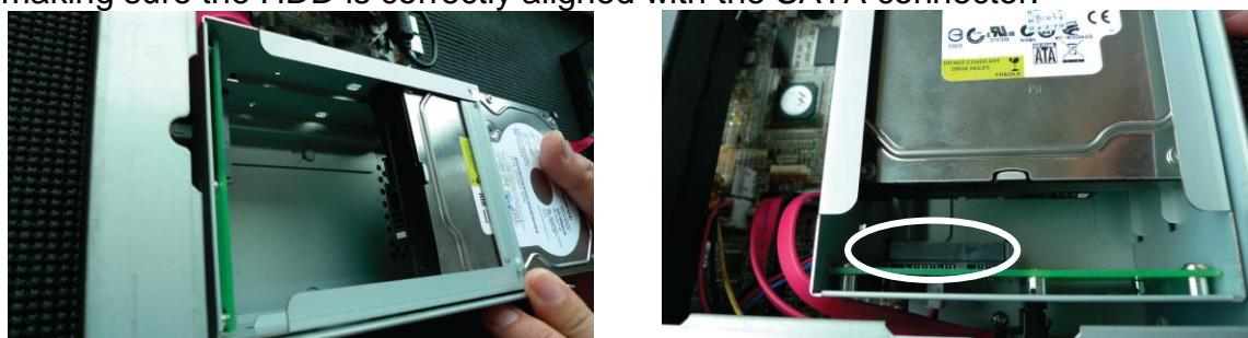
4. Secure the HDD with the screw provided.
