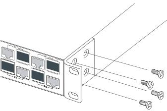
**2.** Mount the device in the rack, using four rack-mounting screws (not provided). Be sure to secure the lower rack-mounting screws first to prevent the brackets being bent by the weight of the switch.
