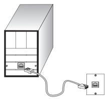
2. If the device is a network card and the switch is in the wiring closet, attach the other end of the cable segment to a modular wall outlet that is connected to the wiring closet. (See the section "Network Wiring Connections.") Otherwise, attach the other end to an available port on the switch.
