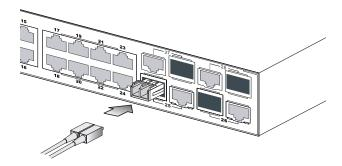
**4.** As a connection is made, check the Link LED on the switch corresponding to the port to be sure that the connection is valid.
