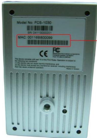
Noted the serial number from the label on the unit. The serial number is the same as Ethernet address.
