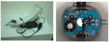
**Step 3:** Screw the camera on the mounting kit. **Step 4:** Screw on the two side screws, and plug in the power to the IP camera.
