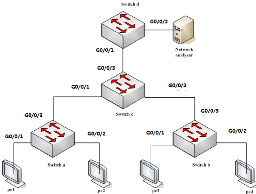
Users need to monitor the flow of the g0/0/1 port in switch a and the g0/0/1 port in switch b at the network analyzer, which can be realized through remote mirroring. The configuration is as follows:
