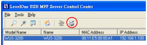
Select USB1 Port or USB2 Port to add the printer in Add the printer box, choose to use host name or IP address to represent MFP server in Select IP Address or Host Name in printer port box, and select the network printing protocol of Printing with Network Path (SMB).
