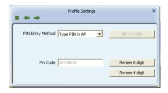
Click "Start PIN" button, then Input the PIN code of the adapter's WPS page into the router's WPS configure page, then click "connect", please wait a moment, the connection between the adapter and the router will be established automatically.
