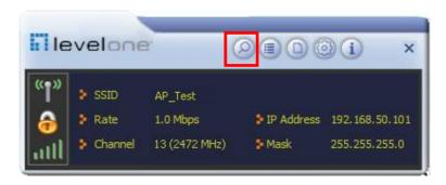
Select Available Network tab and click Refresh button to refresh current available wireless network, you can double click it after highlighting a wireless network you want to connect, If it is encrypted, you need to enter Network Key and confirm it and it will be OK. (Note: profile will detect the Authentication and Encryption of current wireless network, you don't need to change it.)
