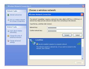
When the highlighted part shows "Connected", it indicates the connection is successful.
