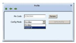
Select "Registrar" as the config mode and enter the router's PIN code, such as 35475088 that displays on the router's WPS screen in section 2.1, in the PIN code field here.
