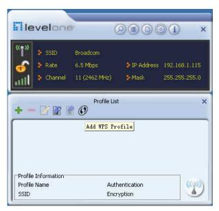
2) On the Profile screen, select "Push-Button Configuration" (PBC) and then click the "Next" button, select "Start PBC" two minutes after the router enables the WPS function. The connection is established when the negotiating process finishes.
