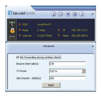
**No forwarding among wireless clients**: This feature isolates the communications among the wireless clients that are connected to the wireless adapter in AP mode.
