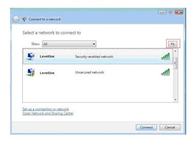
3. If the wireless network that you are connecting has enabled security mode, you'll be prompted to enter the network key .Click "Connect" after you enter the correct key.
