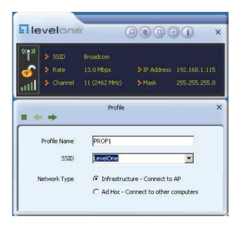
Click the next button to select the authentication type and encryption type such as WPA—PSK and AES, and then input the key and click next.
