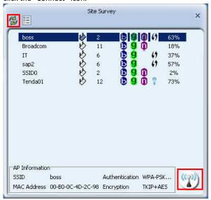
For the networks that are not encrypted, you can directly click "Connect". However, for the encrypted wireless networks,a "Profile" dialog will pop up and you must select the corresponding authentication type and encryption type, and then click the "Next" button to input the correct key. Please note that this type of connection will not create a profile , thus next time connect to this network you still need to select it manually.
