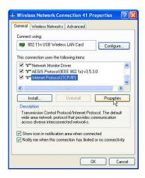
**d.** Please enter the IP address and subnet mask, and make sure this IP address is not used by other devices in the network. For example: if your wireless adapter's IP address is 192.168.0.1, then set other wireless adapters' IP addresses within the range of 192.168.0.2—192.168.0.254. Click
