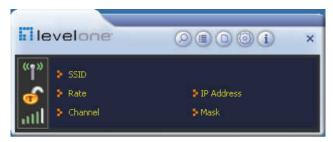
The function buttons on the top(From L to R )are respectively Site Survey, Link Information, Profile, Advanced, About, and MiniSize. While the left column displays Turn On/Off RF, Security /No security, and Signal status.
