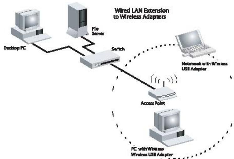
The infrastructure configuration not only extends the accessibility of wireless PCs to the wired LAN, but also increases the effective wireless transmission range for wireless PCs by passing their signal through one or more access points.
