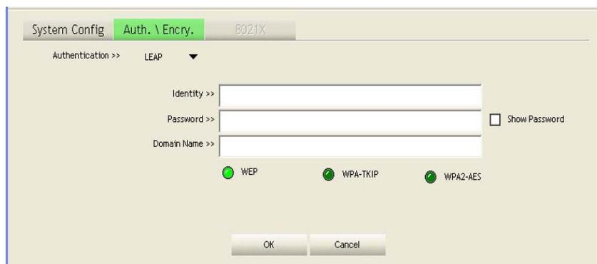
**WPA / WPA-PSK:** Wi-Fi Protected Access (WPA) employs a combination of technologies to provide an enhanced security solution for wireless networks. The WPA Pre-shared Key (WPA-PSK) mode for small networks uses a common password phrase that must be manually distributed to all clients that want to connect to the network.
