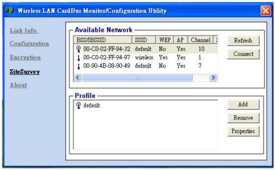
**Available Network** – displays the wireless networks (wireless clients and Access Points) that are in your signal range.
