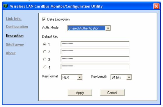
**Encryption:** You can: **Disable or Enable** the WEP data encryption feature. If enabled, it is required to select the **Authentication mode** from the next dropping list.
