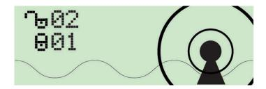
In scanning mode the display will display the total number of both non-encrypted and encrypted Wi-Fi signals detected.
