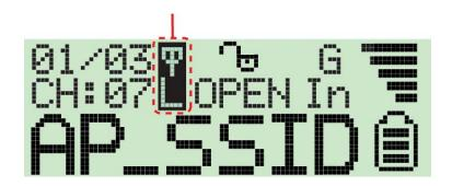
In "lock mode" the detector constantly re-detects and refreshes the signal strength to this specific SSID so the user can move around to find the optimal spot with strongest signal.
