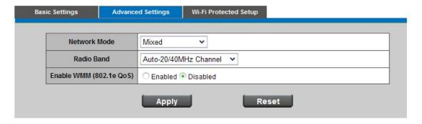
Network Mode - From this drop-down menu, you can select the wireless standards running on your network. If you have both Wireless-B, Wireless-G and Wireless-N (2.4GHz) devices in your network, keep the default setting, **Mixed**. If you have both Wireless-B, Wireless-G devices in your network, select **BG-Mixed**. If you have only Wireless-B devices, select **Wireless-B Only**. If you have only Wireless-N (2.4GHz) devices, select **Wireless-N Only**.
