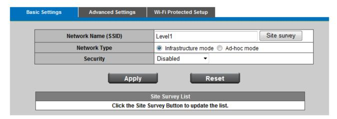
Network Name (SSID) - The SSID is the network name shared among all points in a wireless network. The SSID must be identical for all devices in the wireless network. It is case-sensitive and can be up to 32 characters in length. Make sure this setting is the same for all points in your wireless network.
