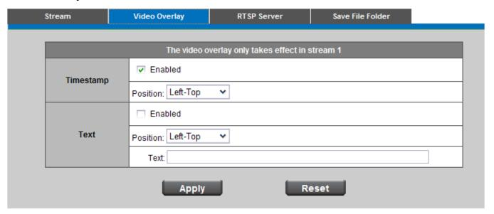
**Video Overlay -** Check to enable the timestamp function and select display position from the drop-down list if user wants date and time to be shown on the screen of the live video. User may also enable and enter the video description in text box; and select display position from the drop-down list if user wants to make a note about the network camera.
