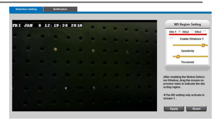
**Detection Setting -** Select and enable the motion detection windows function. Easier to trigger event by higher the sensitivity value and lower the Threshold value.
