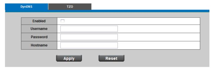
**DynDNS -** Enable the DDNS service allows your Network Camera, especially when assigned with a dynamic IP address, to have a fixed host and domain name. Note that before utilizing this function; please apply a dynamic domain account first. Enter the username, password and hostname when enabled the DDNS.
