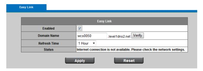
**Easy Link** – the IP camera had bundle with free Level1DNS<sup>™</sup> service that allows user to remote access the IP camera via internet. The default domain name is MAC address, you can also register your own name on-line but it have to check the available first. The status will show the connection with Level1DNSTM service.
