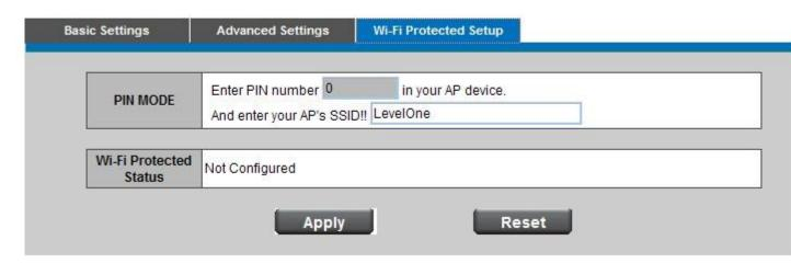
Use this method if your client device has a Wi-Fi Protected Setup PIN number.
