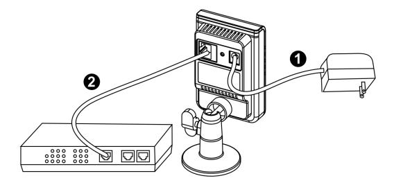
Please check your product package contains all the accessories listed in the foregoing Package Contents. Upon powering up, the power LED will become lighted first and then the device will go through booting process. The status LED will be steady amber for getting IP address. After getting IP Address, the link LED will blink orange while network connection is processing.
