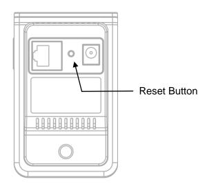
The reset button is used to reset the system or restore the factory default settings. Sometimes resetting the system can return the camera to normal operation. If the problems remain after reset, please restore the factory settings and install it again.
