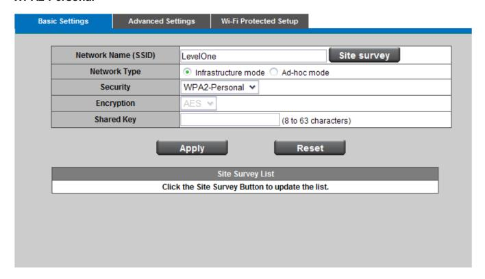
WPA2 supports AES encryption methods with dynamic encryption keys.
