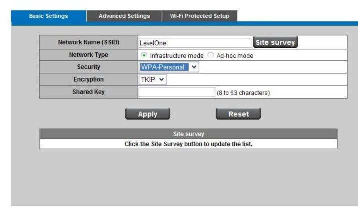
WPA supports two encryption methods, TKIP and AES, with dynamic encryption keys. Select the type of algorithm, TKIP or AES. The default is TKIP.
