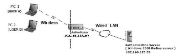
Figure 1: Testing Environment (Use Windows 2000 Radius Server)
