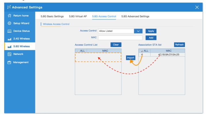
4. After the user's MAC address is added to the access control list, Click Apply. After setting is completed, it will start to allow users access to this wireless AP function
