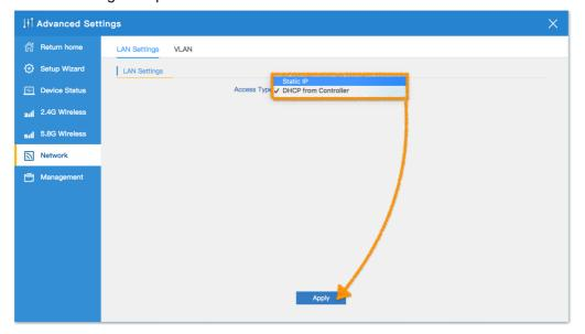
5. Sample Static IP mode setting method, then click Apply to continue. (Please contact with ISP for correct IP address, Subnet MasDNS address)
