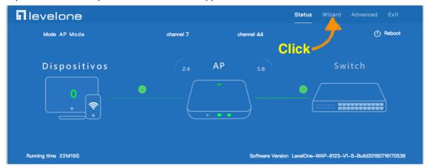
2. Wizard: It instruct users to configure wireless AP's operation mode based on needs: there are four operation mode including gateway, repeater, WISP, Wireless AP. Please confirm the operation mode first before configuration starting.
