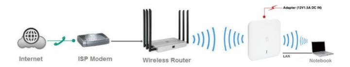
AP Mode: Please Make sure that the upper device has a router, Only after confirming can use AP Mode
