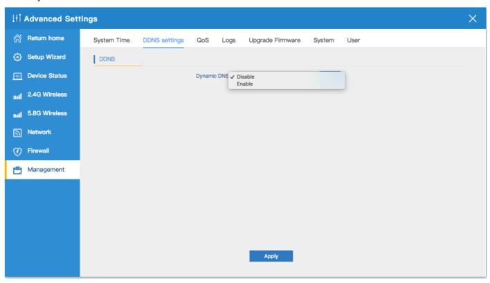
2. For users no apply for an ISP fixed IP address, only Floating real IP address, you can also connect to the network device in WAP-8123 through the DDNS service.
