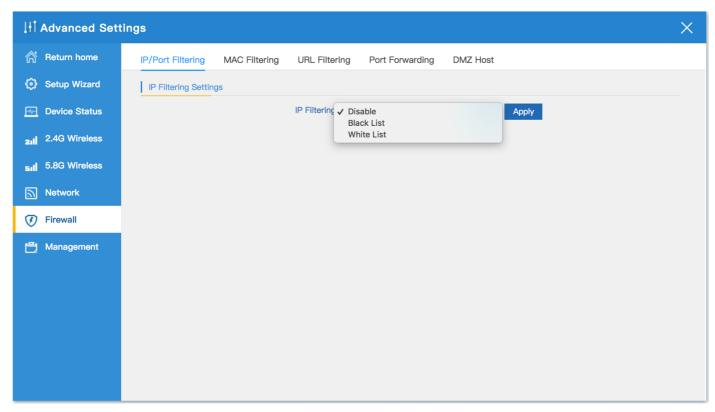
**2.Black List :** IP Address that can be specified as a separate or range , and then specifies the port range  $(1\sim65535)$  and protocol(TCP/UDP).
