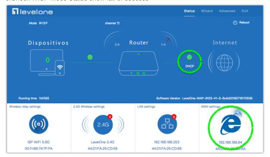
7. Check WISP Mode data for WAN Status, Check IP address that is received by DHCP.
