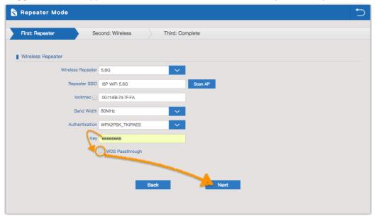
4. If choose to relay the front-end 5.8G wireless signal to extend the wireless signal range. Can choose to enable or disable the 2.4G wireless broadcast of the WAP-8123 itself.
