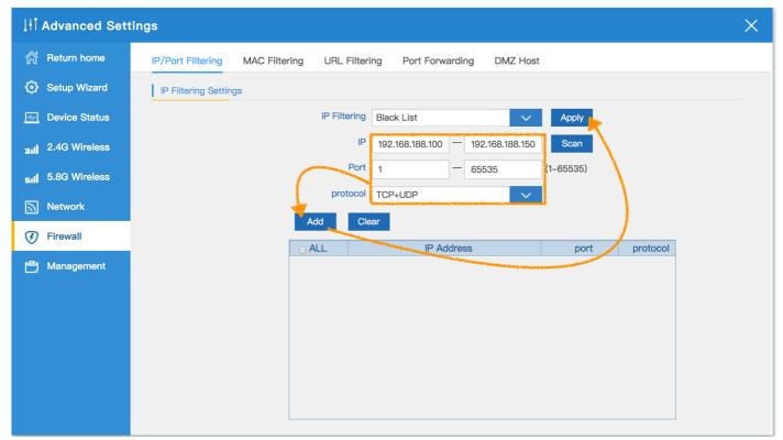
**3.White List**: IP Address that can be specified as a separate or range, and then specifies the port range (1~65535) and protocol(TCP/UDP), which is set as the status of the allow.
