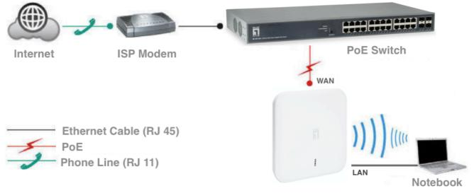
WISP mode: Receive ISP Modem Wireless network and select one of them Internet access method (PPPoE, DHCP, static IP).
