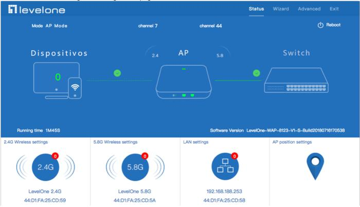
2. Then in Wireless Setting, GUI configuration page showed as below: User can configure the SSID, password, band width, channel here, then Apply to finish.
