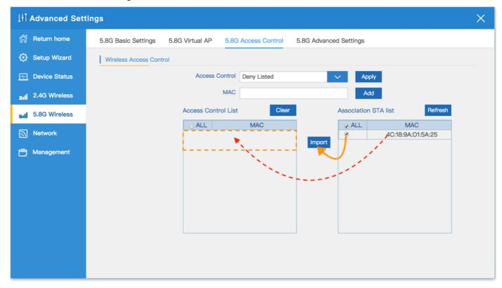
6. After the user's MAC address is added to the access control list, Click Apply. After setting is completed, it will start to deny users access to this wireless AP function
