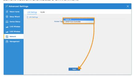
2. Use DHCP for Controller mode, please confirm that the current network architecture has IP address allocation.
