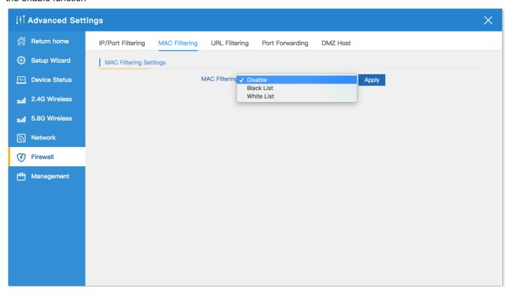
**2.Black List:** Scan specified mode or manual input mode to set, you can block the specified MAC address to connect to the Internet, leaving only link Regional network function.
