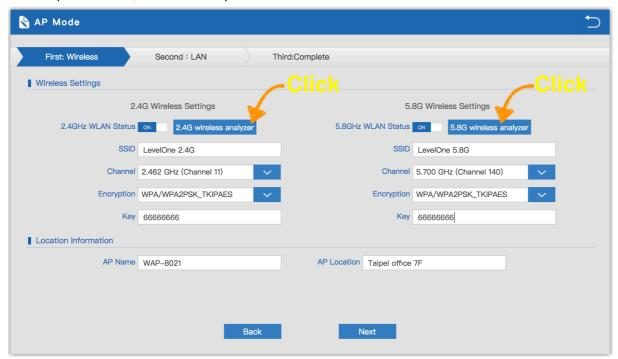
2. Wireless analyzer Look for Unoccupied channel (2.4GHz)
