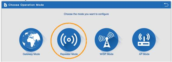
1.Can choose to relay the front-end 2.4G or 5.8G wireless signal to extend the wireless signal range. Select the AP's SSID want to bridge, take "wireless 2.4G" for example, then input the AP's key, click Scan AP
