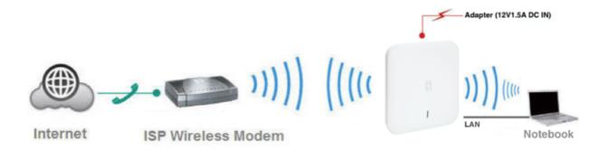
Repeater mode: The WAP-8123 can bridge and extend the existing WiFi signal in this
