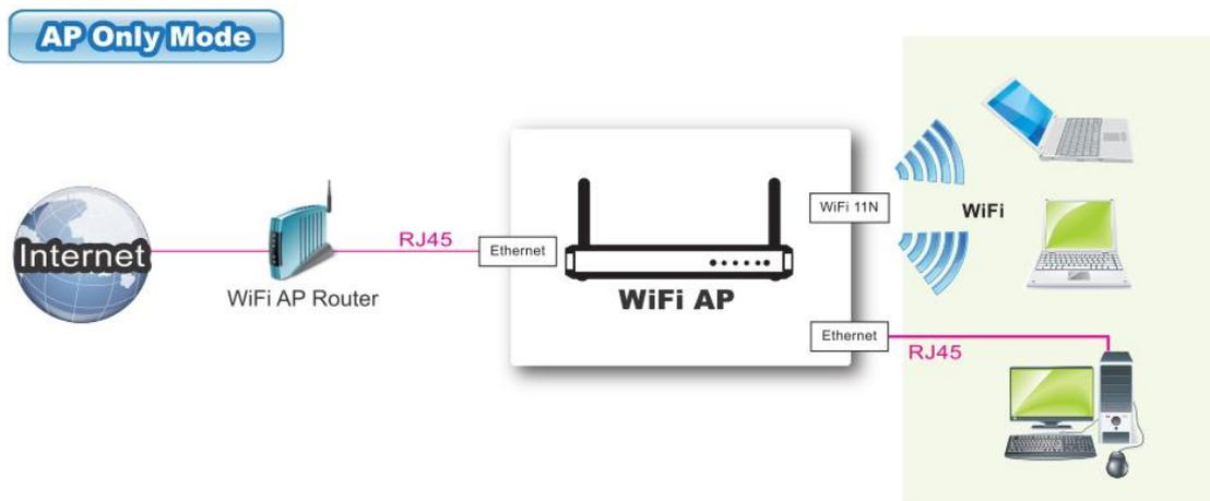
When acting as an access point, this device connects all the wireless stations to a wired network.
