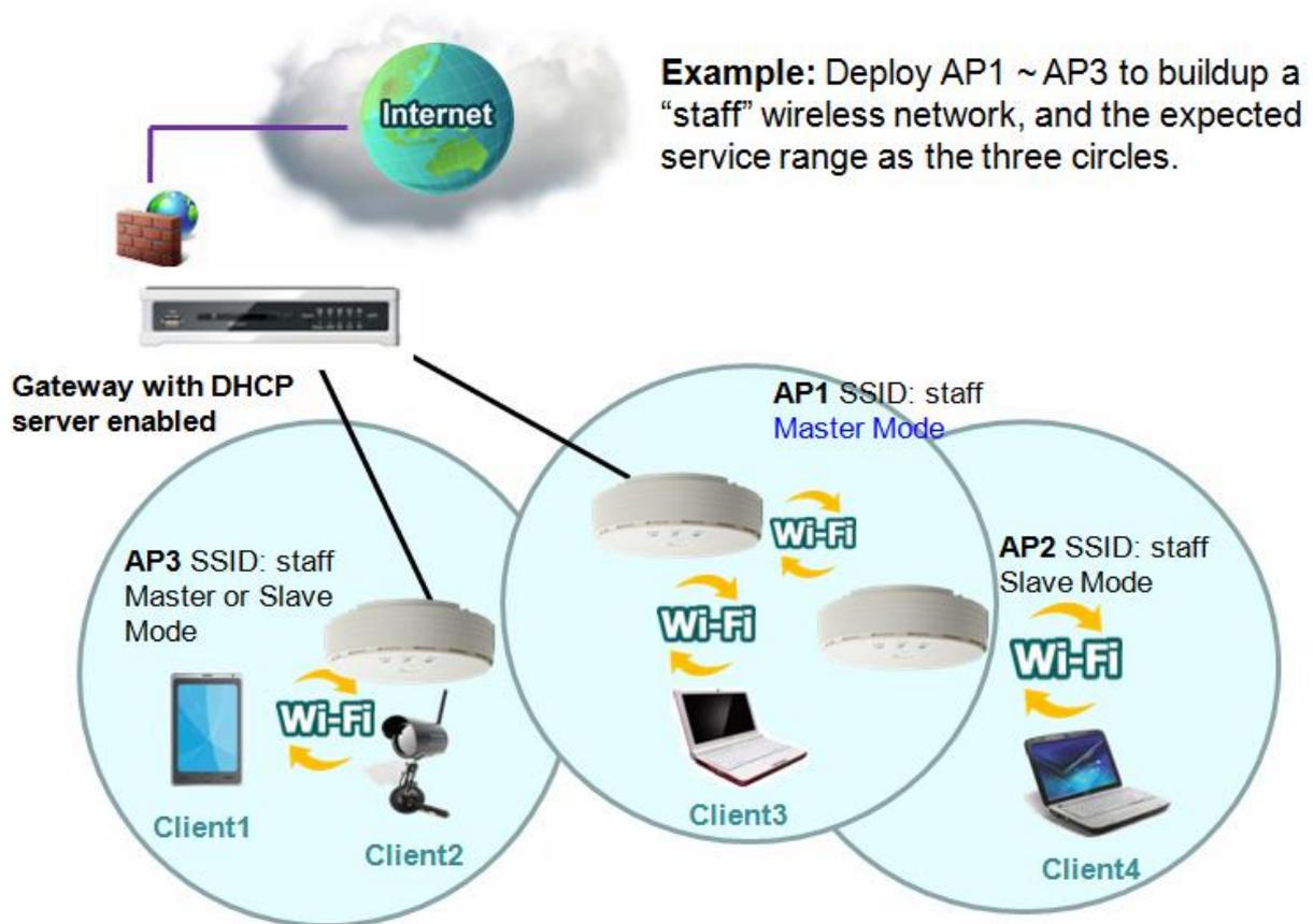
**Example:** Deploy AP1 ~ AP3 to build up a “staff” wireless network, and the expected service range as the three circles.
