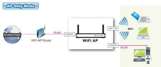
When acting as an access point, this device connects all the wireless stations to a wired network.
