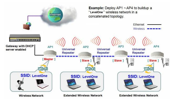
As illustrated in above figure, if you intend to deploy 4 APs (AP1 ~ AP4) to create a "LevelOne" wireless network, you can follow the procedure below:
