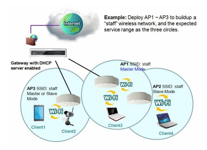
As illustrated in above figure, how to configure the three APs (AP1, AP2, AP3) to build up the "staff" wireless network? You can follow the procedure bellow:
