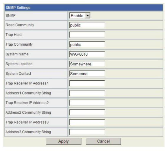
This device is compatible with SNMP v1/v2c and provides standard MIB II. Currently only the "public" community string is available and the modified settings by SNMP SET request will be lost after rebooting the device
