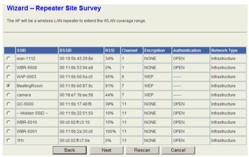
In the second page, setup the wireless encryption to associate the target AP. You must know the encryption/key of the target AP before you setup here.
