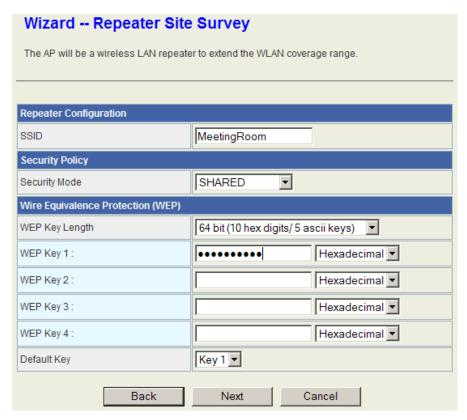
In the third page, setup the WLAN of the device for the other clients to connect.
