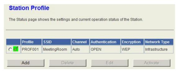
In the first page, you can see the profile list to show the information including Profile name, SSID, Channel, Authentication, Encryption and Network Type. Use four buttons to manage the profile list. The "Add" button is to add a new profile. The "Delete" button is to delete the selected profile. The "Edit" button is to edit the selected profile. The "Activate" button is to enable the selected button, so this device will associate to the AP according to the profile.
