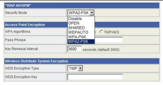
The available options show according to the numbers of the BSSID in the Basic Setting. Each SSID can setup different encryption type. For example, set up 4 BSSID and 4 sets of security shows on this page:
