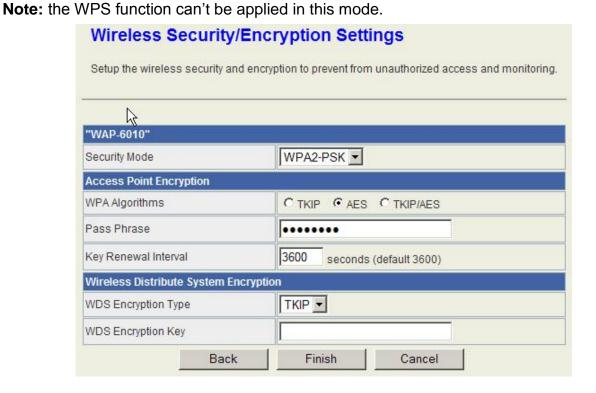
**Repeater Mode:** Setup Wizard will guide you through Repeater Site Survey, Repeater Site encryption, Wireless Basic Setting and the Wireless encryption pages. In this mode, this device plays two roles, one is a Client/Station to associate the target AP, and the other is an AP to allow the WLAN client/station to associate into. Therefore the WLAN of this device is bridged to the WLAN of the target AP.
