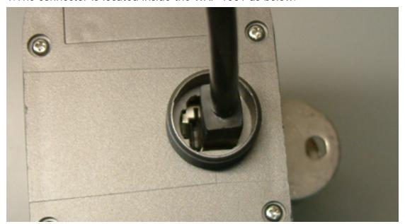
2. Insert the flat screwdriver and make sure that RJ45 connector is compressed.
