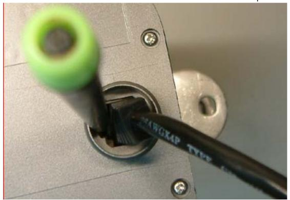
3.At this moment, the screwdriver should compressed RJ45 connector like the picture below inside the WAP-1001.
