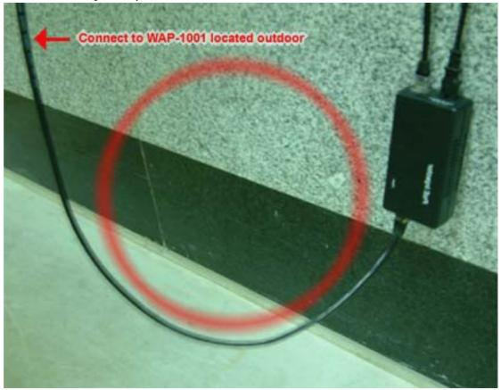
In order to avoid the problem mentioned above, please place the POE injector higher than the Ethernet cable, so that the raindrop will not permeate the POE injector.
