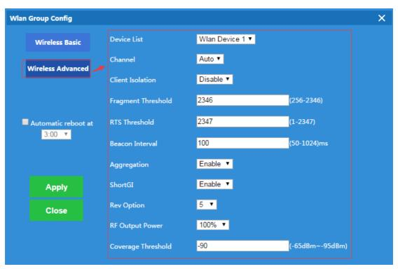
Channel: Auto in default, but recommend to setup channel by manual based on environment.
