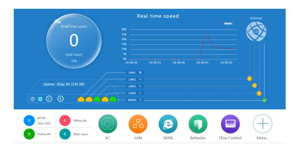
RealTime Users: Mean the QTY of end users access into it when it work as Gateway.Link Count: Mean the QTY of internet link.Real time speed: Mean the WAN Ethernet speed
