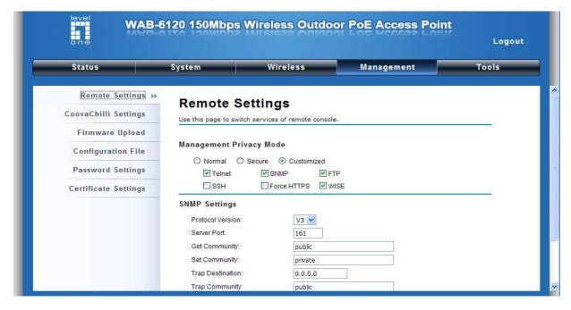
**Figure 35 SNMP Configuration**
