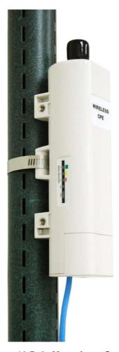
Figure 10 Pole Mounting – Step 3
