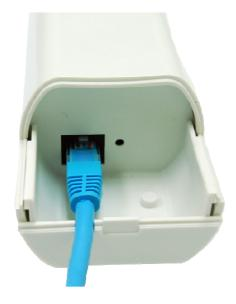
**Figure 4 Cable Connection**
