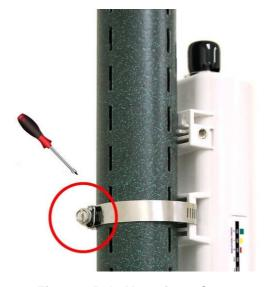
Figure 9 Pole Mounting - Step 2
