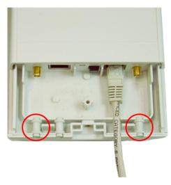
2. Connect your external antenna to the SMA-type connectors at the bottom of the CPE.
