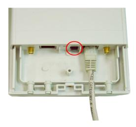
6. Attach and fasten the removable cover to the bottom of the unit with the screw.
