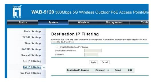
Figure 17 Destination IP Filtering
