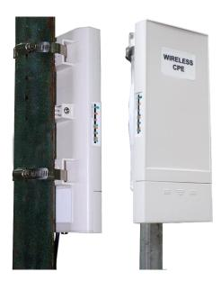
Figure 8 Pole Mounting - Step 2
