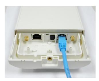
**Figure 4 Cable Connection**
