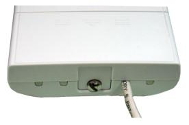
7. Power on the WAB-5120 300Mbps 5G Wireless Outdoor PoE Access Point/Bridge by plugging the power adapter to the power socket.
