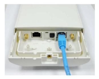
Figure 4 Cable Connection
