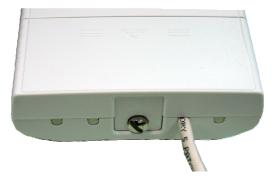
Power on the WAB-5120 300Mbps 5G Wireless Outdoor PoE Access Point/Bridge by plugging the power adapter to the power socket.
