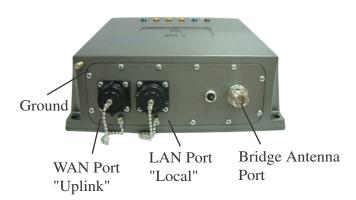
Ethernet cable is thus run from the WAB–2000 to the power injector which is then connected to a power source and the wired LAN. A second (LAN Port) Ethernet connector is designed for use during initial configuration only. This uses an RJ45 cable to connect the WAB–2000 to a laptop. The following diagram demonstrates the setup.
