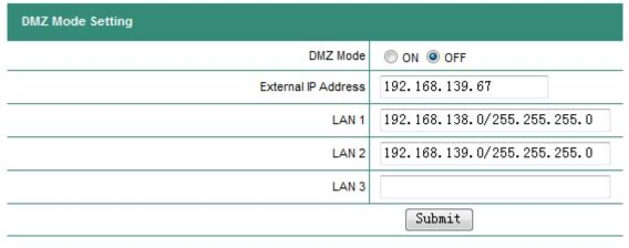
The DMZ must be set ON if the DMZ of firewall is activated.
