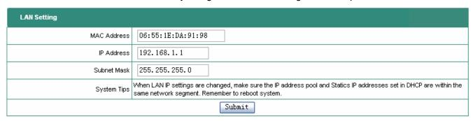
MAC Address should be unique in the same network, and IP Address must be in the format of xxx.xxx.xxx and xxx is from 0 to 255, e.g. 192.168.1.1. Subnet Mask is used for network segmentation. Please make sure the mask is correct and all the VoIP devices are within the same network as Embedded IP-PBX.
