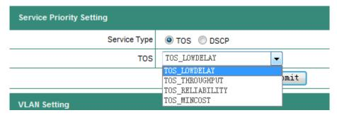
DSCP field is a superset of TOS, its definition is backward-compatible with TOS, and its value can be from 0 to 63, with 0 for minimum priority, 63 for max priority.
