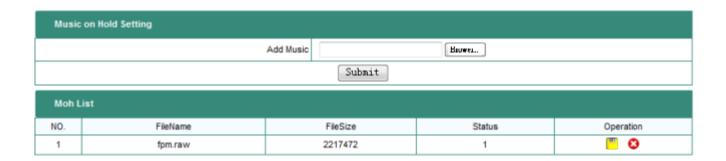
Music ON Hold requires a unique file format, and any MP3 files must be converted to **.raw** format before upload to Embedded IP-PBX for use of Music ON Hold.
