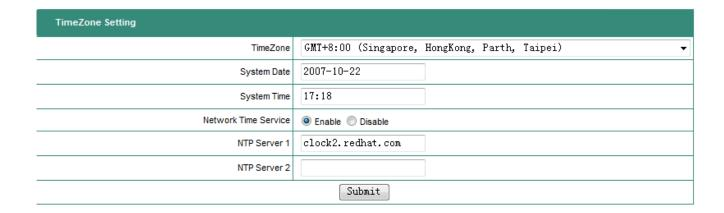
Press **Submit** to save the configurations, and press **Reboot** to activate the new configurations.
