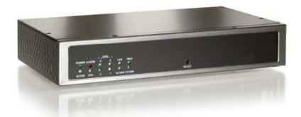
The Embedded IP-PBX is an embedded Voice over IP (VoIP) PBX Server with Session Initiation Protocol (SIP) to provide IP extension phone connections for global virtual office of small-to-medium business (SMB) companys. Equipped with 4 x FXO ports, Ethernet LAN and WAN ports plus Life Line features, Embedded IP-PBX integrates the telephony network and the data network into a manageable converged network to provide an efficient and economical PBX for global long distance voice communications.
