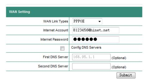
When Embedded IP-PBX connects to ADSL Modem with PPPOE link, you need to enter the account name and password for PPPOE. In addition, you may select the DNS server and enter the IP address for the First and Second DNS servers.
