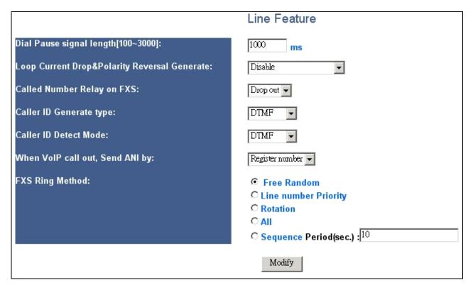
/VoIP Setup/Line Configure/ Line Feature
