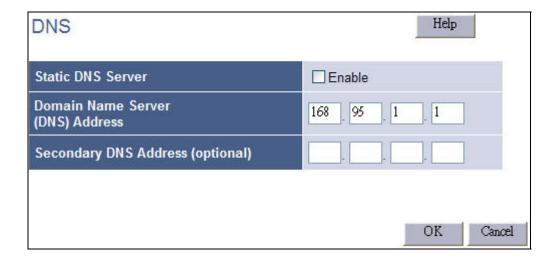
This page sets the primary and secondary DNS servers, which were given by your ISP or known to you. When a domain name request received, the gateway tries to resolve to it from the Primary Domain Name Server. Resolving failed, the gateway tries the Secondary sever again.
