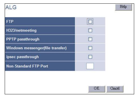
Some applications have to do Application Level Gateway (ALG) to monitor the transaction or monitor the payload of the packet. This page let you setup them.
