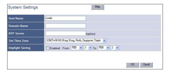
This page is used to configure the names given by the ISP, if any, to represent the gateway, and also to set the local time zone.
