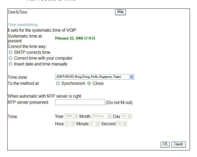
This page is used to setting the system time of VoIP gateway; it can define the correct time by which ways.
