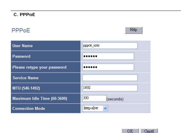
This page is the PPPoE configuration page. Most of the ISPs request the user to connect to central office (CO) side via PPPoE, acronym of Point-to-Point Protocol over Ethernet, which provides authentication, authorization and accounting.
