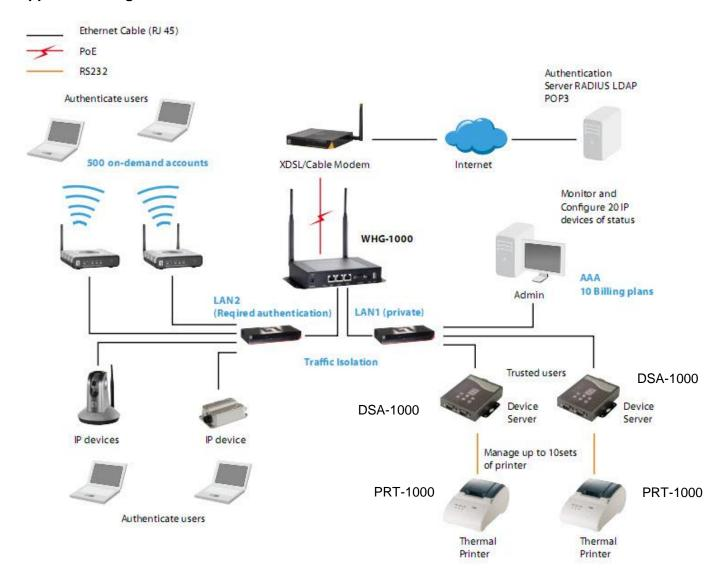
Though DSA-1000 is specifically designed to for on-demand account generation and operate Thermal Printers, it can also be deployed independently to connect other RS232 devices to an Ethernet network for remote operation. If you will be deploying DSA-1000 independently to manage other serial devices, please carefully set the *Serial Settings* in DSA-1000 to match the operating needs of your serial device.
