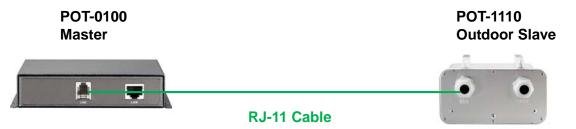
3. Connect the LAN port of POT-1110 (Outdoor Slave) to power up the PD device as the following connection.
