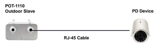
4. Power on PSE Source. POT system will start handshaking .When LINE LED is always on, The POT system is connection ready.
