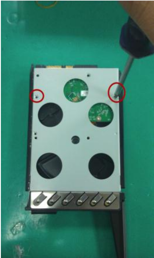
Place the HDD in the tray and
