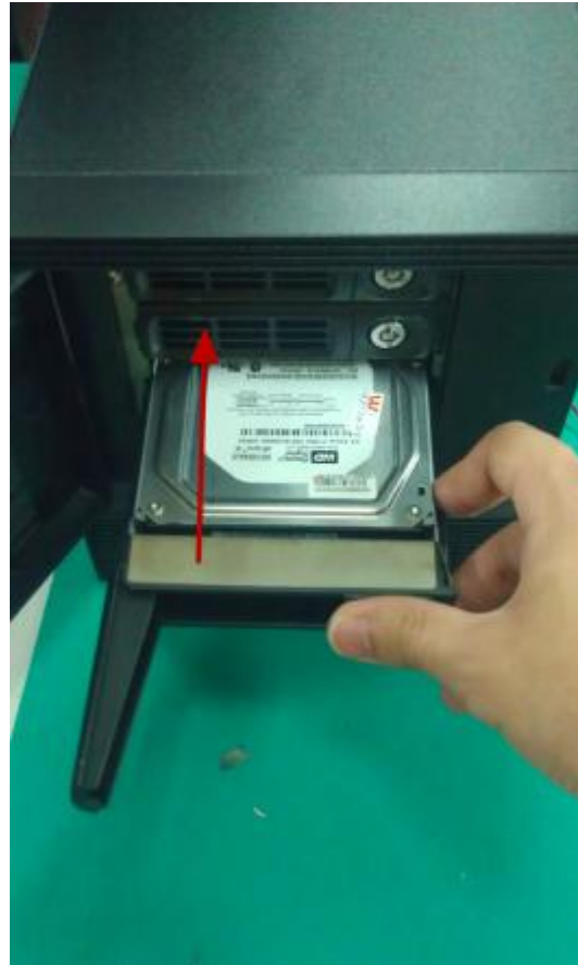
Put the HDD tray back to the case. Secure it with the screws at the bottom of the tray
