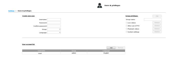
Multiple users can access the recorder simultaneously. You can add, remove, and edit users by using options provided in this page to keep user information organized. Each recorder comes with a built-in
