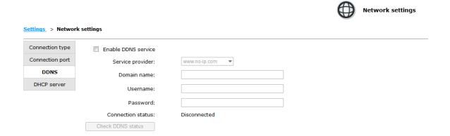
DDNS, which stands for "Dynamic DNS", is a method, protocol, or network service that provides the capability for a networked device, such as a router or computer system (in this case, the NVR) using the Internet Protocol Suite, to notify a domain name server to change, in real time, the active DNS configuration of its configured hostnames, addresses or other information stored in DNS.
