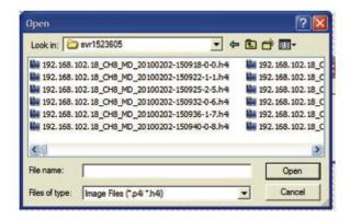
The NVR sends snapshots that are taken when an event occurs to a destined FTP server or mail recipient. These types of snapshot images are saved in a proprietary image file format, h4i or p4i, and can only be opened by the NVR media player.
