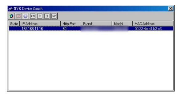
The NVR should be located and its IP address should be displayed.
