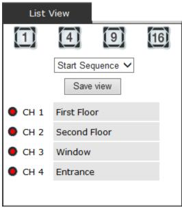
It displays the list of channels added to the NVR. Each channel represents a camera with its name, the channel number and its currents status.
