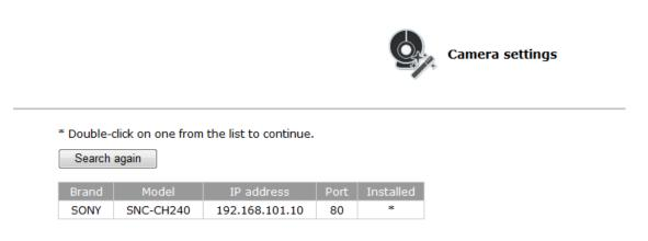
\*If cameras are marked with "\*" in the search result, it means those cameras are already configured and connected to the NVR.
