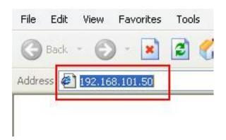
The PC that is connected directly to the NVR (or within the same local area network) should receive an IP from the NVR. Simply access the NVR from your web browser with its IP address
