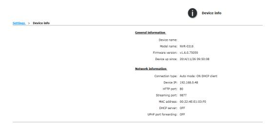
Device info gives users a glance of the overall system status and allows users to perform maintenance tasks such as upgrading firm- ware, restore/backup device settings or reboot device ....etc.
