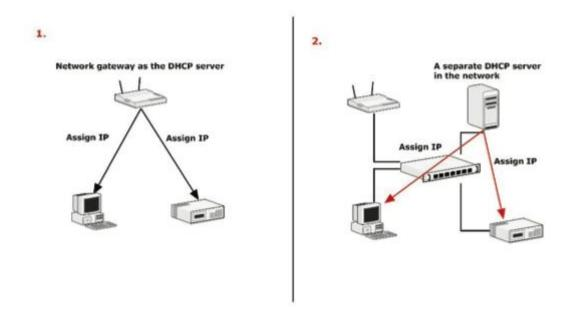
If the NVR is placed in a corporate network or a local area network where a DHCP server is already presented, run the "NVR Search" utility from a computer that is on the same network and locate the NVR with its IP address that is assigned by the top-level DHCP server.
