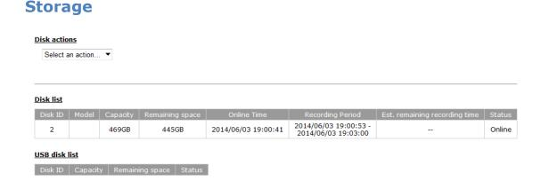
Once you install a hard disk to the recorder, you would need to initialize it so that it can be ready for recording. You can obtain basic information about the disk you installed in this page.
