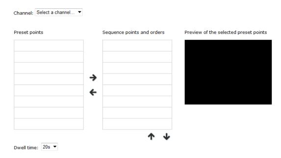
Once you have multiple preset points defined for a camera, it is convenient for monitoring to set up the sequencing viewing among those preset point and let the recorder automatically switch between them for you.
