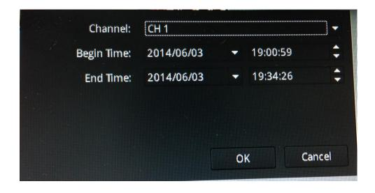
On local UI, the recorded video can be backed up to a USB disk with AVI file. It is required to plug in a USB disk formatted in FAT32 prior to using the backup function. Click "OK" to open a pop-up dialog for USB disk options
