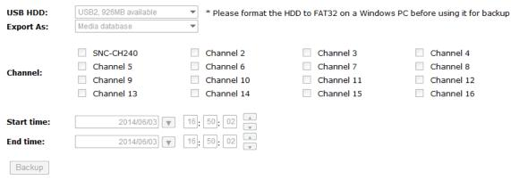
It's a function that allows users to backup the recording data in its database file format as well as in AVI to the externally connected USB hard disk.
