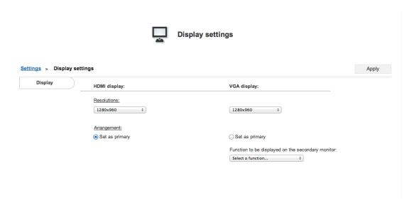
The "Display" configuration page allows you to choose the most optimized display resolution for the monitor that's used with NVR, as there will be circumstances that the incorrect resolution may be used when the system first boots up.
