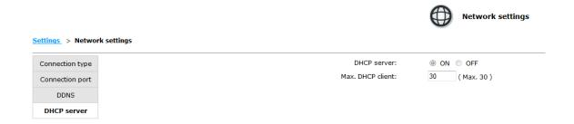
The built-in DHCP Server function is NOT always configurable and is greatly dependent to the connection type that is set to use in "Network Settings".
