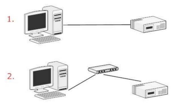
The NVR comes with a pre-configured static IP "192.168.101.50". However, it is only used when there is no DHCP server presented in the network. The NVR will turn on its DHCP server function and act as the DHCP server in the network. To connect to the NVR, use a PC that is on the same network over a switch or hub, or connect the PC directly to the NVR using a crossover CAT5 Ethernet cable.
