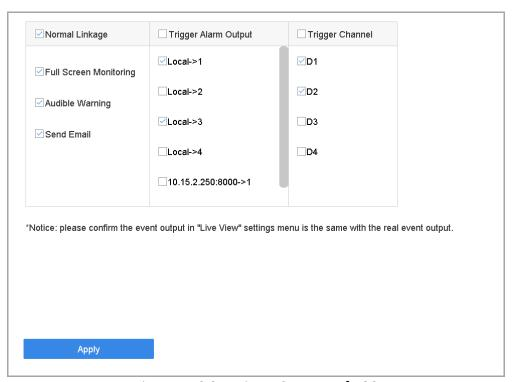
Figure 14-8 Set Trigger Cameras of POS
