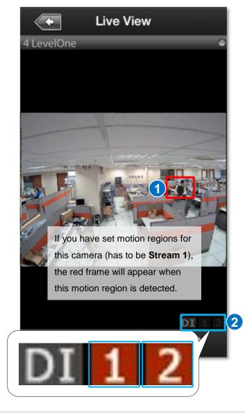
Once the connected DI device is triggered, the DI number will appear in orange. You have to make sure the DI device has been well connected and configured with the camera first.
