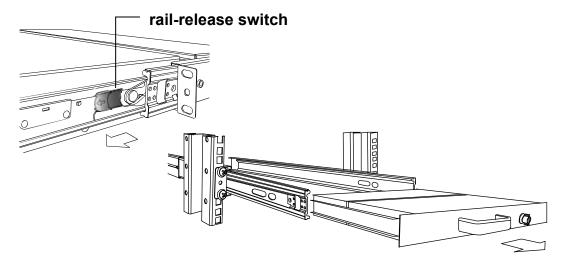
1. Push rail-lock switch on the rail and push rail back.(Both sides)
