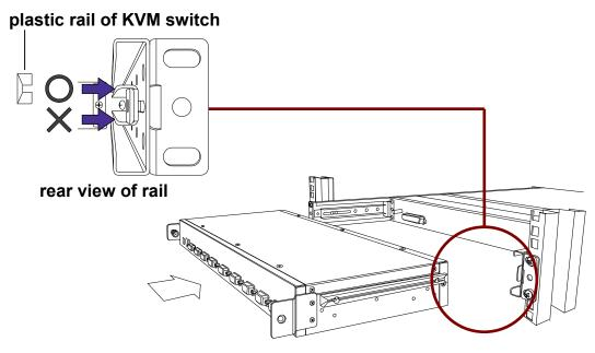
3. Tight thumb screw of bracket A up to fix KVM switch in console and finish installation. (Both sides)
