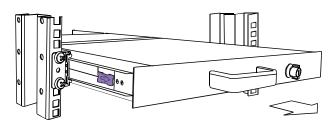
5. Pull rail-release switch and pull console out.(Both sides. Be careful when pull out console.)
