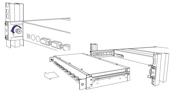
2. Release three screws in rear of the console. (Both sides)
