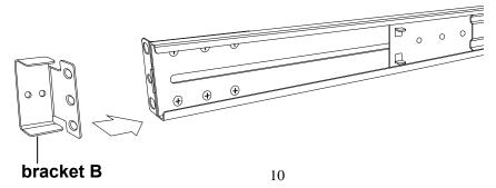
4. Install four screws (don't tight-up) to combine rail, bracket B and bracket C.
