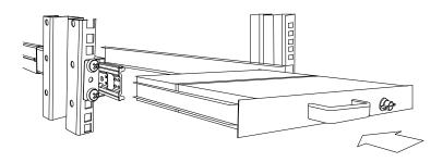
8. Unlock and pull rail-lock switch (left and right at the same time) then push console to the end.
