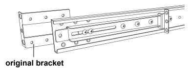
4. Adjust rail and input bracket A to rear of the rail then adjust bracket A to fit your cabinet. Install 2~3 screws (don't tight-up) upon the length you need. One is forbidden.
