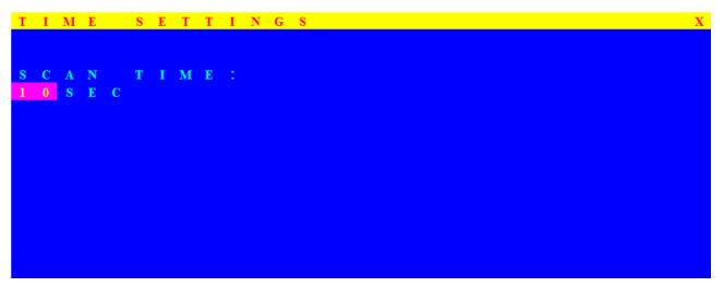
When the Auto-Scan function is activated, the KVM switch will auto-scan the host ports one by one in the interval as setting. Notice that the port without connecting to a computer/server will be skipped over on the scan. The interval range is 5 ~ 99 seconds, and the default interval is 10 seconds. Press "**Enter**" key to save the SCAN TIME setting.
