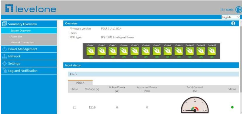
Select **Inlet Configuration** from the Power Management menu. The Inlet Configuration page displays as shown.
