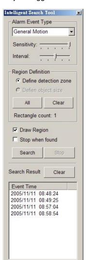
**Stop when found**: Check the box, and the video will stop at the point when a motion in the detection zone is detected. Otherwise, the video will keep rolling and all the events detected will show on the list in Search Result box. Click on the listed event date/time, you will jump to the point in the video where a motion is detected.
