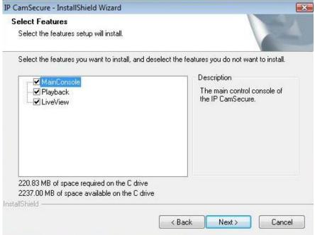
*Hint:* For example, select only Playback and LiveView for installation. Install and use only these features on multiple remote sites at home or anywhere with a PC.
