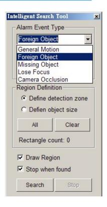
**Define detection zone**: To detect Foreign Object you have to define a detection zone. Left-click and drag, draw a detection zone. Alarm will be triggered when an object appears in the detection zone.
