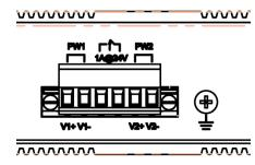
To make power connection – Follow the printed polarity for V1+, V1-, V2+, V2-, and ground. Connect positive wire to V+, connect negative wire to V-, also connect neutral wire to the ground screw as shown.
