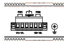
To make power connection – Follow the printed polarity for V1+, V1-, V2+, V2-, and ground. Connect positive wire to V+, connect negative wire to V-, also connect neutral wire to the ground screw as shown.
