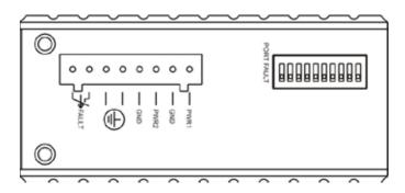
Field Wiring Terminal: Use Copper Conductors Only, 60/75°C, 12-24 AWG torque value 7 lb-in.
