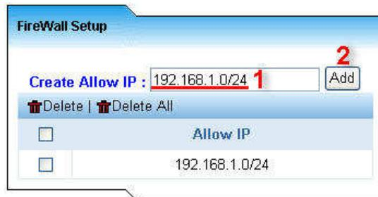
The screenshot shows the 'FireWall Setup' window. At the top, there is a 'Create Allow IP' section with a text input field containing '192.168.1.0/24' (marked with a red '1') and an 'Add' button (marked with a red '2'). Below this, there are 'Delete' and 'Delete All' buttons. A table lists the allowed subnets:
