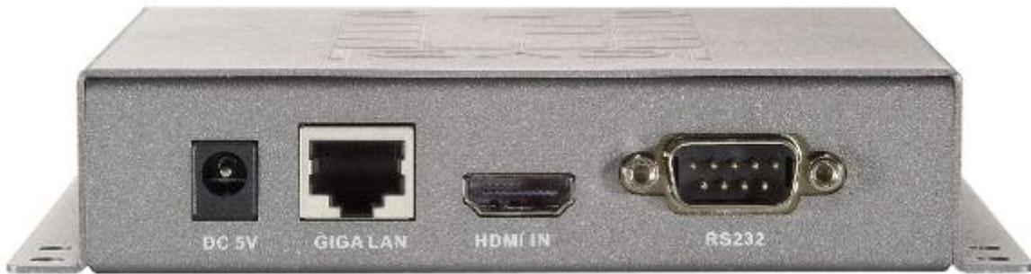
1. **DC5V:** Connect it to the external AC adapter which plugs into an electrical outlet. Or via 802.3af PoE PSE to GIGA LAN port.
