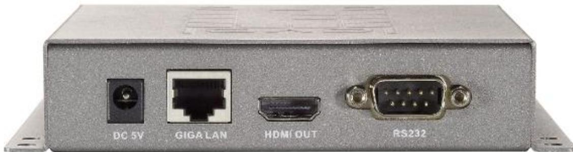
1. **DC5V:** Connect to the supplied AC adapter and plug into an electrical outlet.
