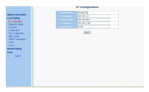
The OAM Media Converter embeds a DHCP client. We could enable/disable this function through the page. If we disable DHCP, we should set the IP, gateway, subnet mask by self, and otherwise, these could not be set. They
