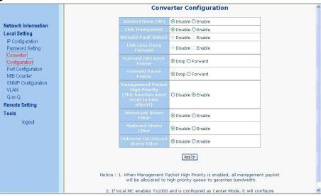
Jumbo Frame (9K): If enable this function, the media converter could pass the max 9KB packet.
