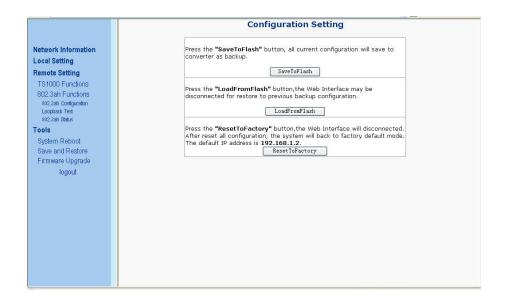
**Backup:** Save local configuration to flash. **Restore:** Restore last saved configuration. **Factory:** User factory default setting.
