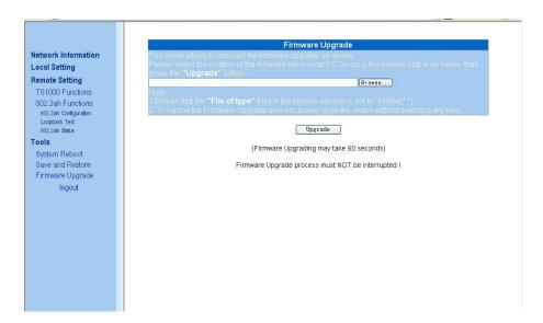
In this page, user could update the firmware by the web browser. User could click the browser button, select the new firmware image file, and then the new code image will be burned into the flash, and reset the device to use the new firmware.
