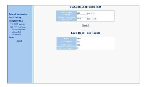
This page could start 802.3ah loopback test. User could configure packet length and packet number.
