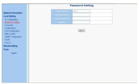
In this page, we could change the password. The password must be 'a'-'z', 'A'-'Z', '0'-'9' and ' '.
