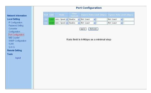
This page could set local device's port status, including work mode, flow control ability, ingress and egress rate limit. There are some predefined rate settings. If user needs some special usage, you could input the rate by self. Because the rate limit is 64kbps as a minimal step, the input rate should be divided exactly by 64. If the value input is not divided exactly by 64, for example 65, the program will be change the rate to 64 automatically.
