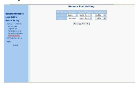
In this page, user could enable/disable remote device's UTP port, change remote device port's speed & duplex and flow control ability. Fiber port should not be disabled.
