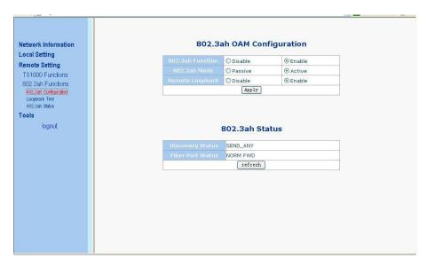
This page could set 803.ah OAM function. User could enable/disable 802.3ah function and set its mode as passive or active mode.
