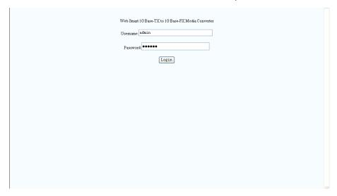
We must input the correct the password to login the web, otherwise we could not access any web pages. The default Username is admin and the default password is 123456 and could be changed in the web. If we don't have any operations in 15 minutes, we need login again.
