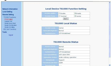
This page could enable/disable TS1000, and set the TS1000 as center mode or terminal mode. If TS1000 is enabled, the TS1000 information will be displayed in the web. And if it's in center mode, and remote device is in terminal mode, remote TS1000 information will also be shown in the page.
