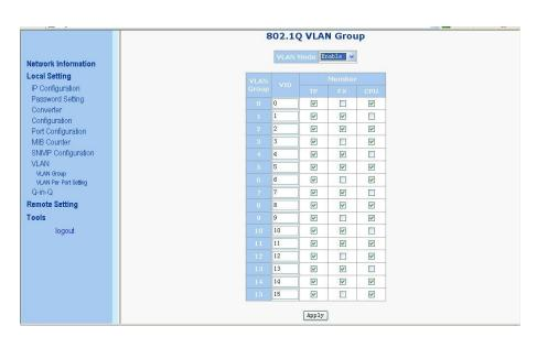
If enable VLAN functions, user could set 16 VLAN entries. Each VLAN entry could set VID and member port. The VID should be 1~4094.
