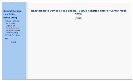
Through TS1000 function, we could let remote device do hardware reset. This function need both devices enable TS1000, local device in center mode and remote device in terminal mode.
