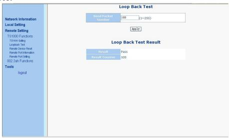
This page could start TS1000 loopback function. User could set TS1000 loopback packet number. After click the "Apply" button, the loopback result will be displayed in the web.
