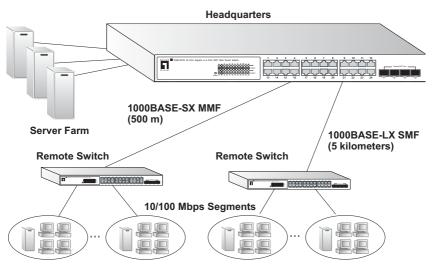
Figure 2-3 Remote Connections with Fiber Cable
