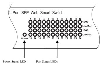
Figure 1-3 Port LEDs and Power LED
