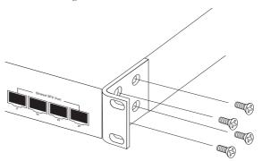
Figure 3-2 Attaching the Brackets
