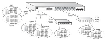
Figure 2-4 Making VLAN Connections
