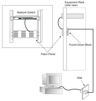
Figure 4-2 Wiring Closet Connections
