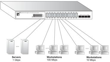
Figure 2-1 Collapsed Backbone
