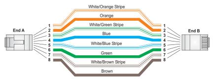
Figure B-2 Straight-through Wiring
