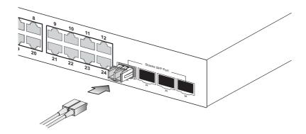
Figure 4-3 Making Connections to SFP Transceivers
