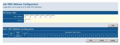
Figure 5-13 Static MAC Address Configuration
