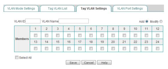
Figure 7-6 Tag-based VLAN Settings
