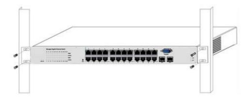
Figure 2-1 Installing the Switch in a Rack
