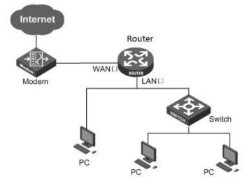
Figure 2\_5 Establish a connection to LAN and WAN
