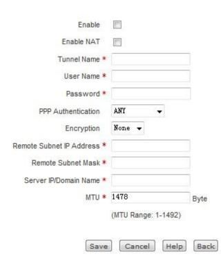
Figure 12\_10 PPTP client Settings
