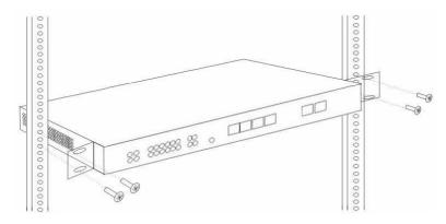
Figure 2\_4 Product rack installation drawing II
