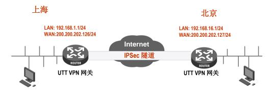
Figure 12\_20 Gateway to gateway topology
