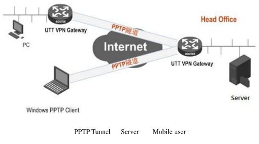
Figure 12\_1 PPTP typical application
