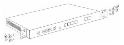
Figure 2\_3 Product rack installation drawing I
